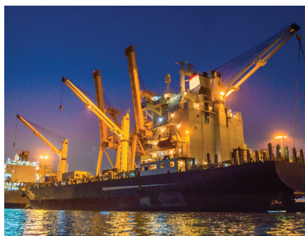
A heavy-lift vessel specifically designed for the carriage of heavy project cargo. Two cranes allow for tandem lifts.
